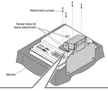
When installing the stand to the monitor, insert the guides of the stand into the guide holes on the monitor to place the stand on the correct position. Then fix the stand firmly with the attachment screws.
